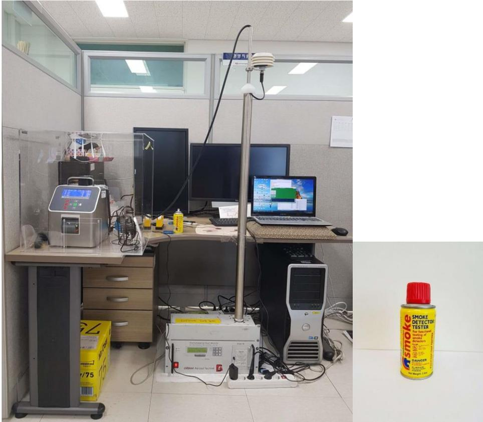
Figure 1. Evaluation environment setup. Piera-1 was placed in close proximity to the 11D's air intake hose. The test spray used in the testing is shown on the right.
