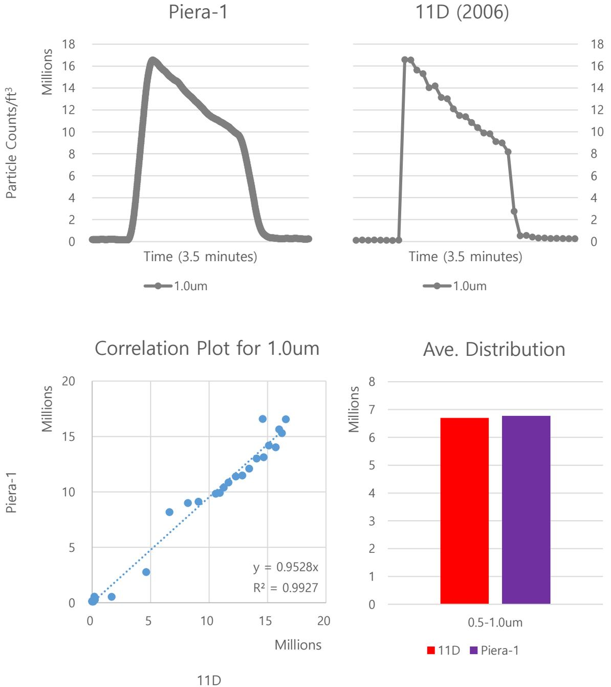
Figure 5. Differential particle count plots for 1.0um, from Piera-1, and 11D with correlation curve and average distribution.
