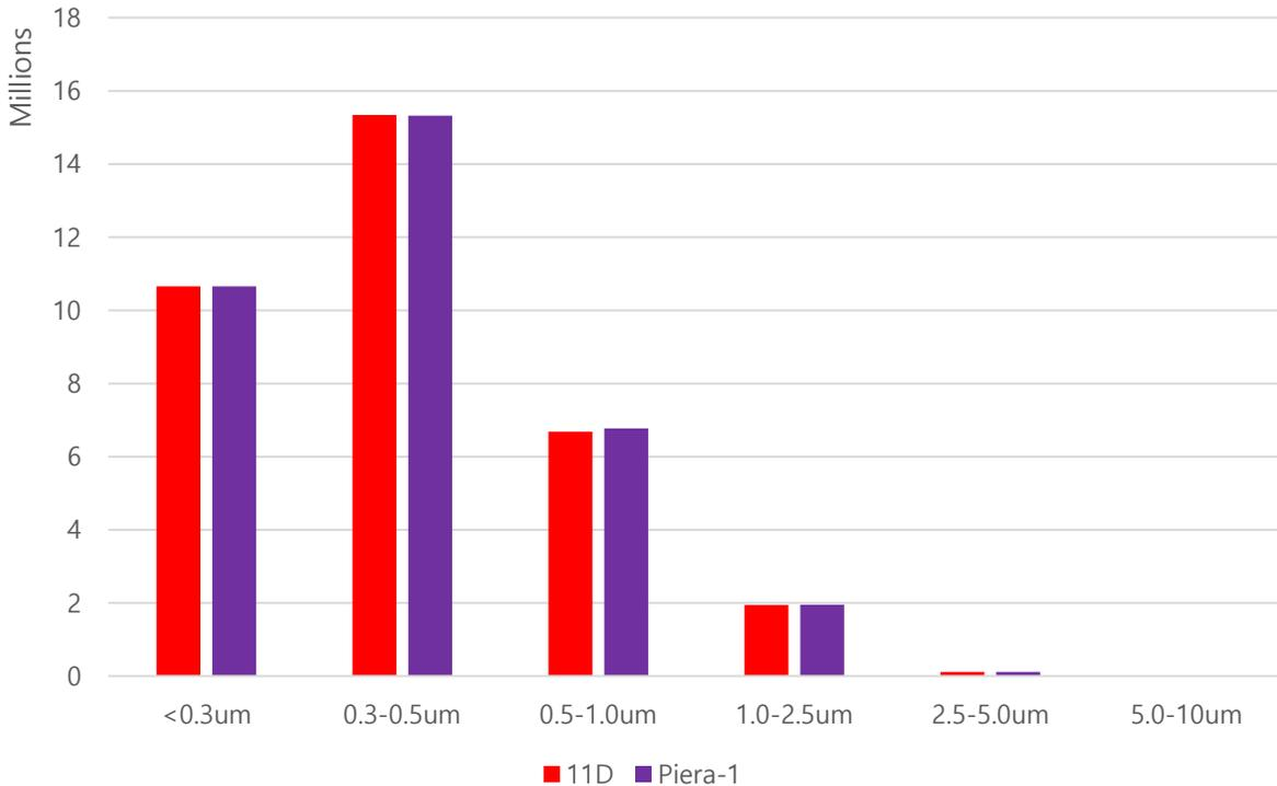
Figure 9. Average differential particle count histograms for all available bins from Piera-1, and 11D.
