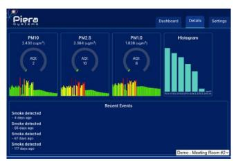
SenseiAQ™ Software displays the data on a dashboard including Air-Quality-Index (AQI) Scores, alerts for vape, smoke, etc. from particle count and distribution. An API supports third party integrations such as Air Quality Management Systems, Air Purifiers, etc. SenseiAQ is an app that runs on Windows, MAC, Android devices or on a cloud service. iOS Support is planned.
