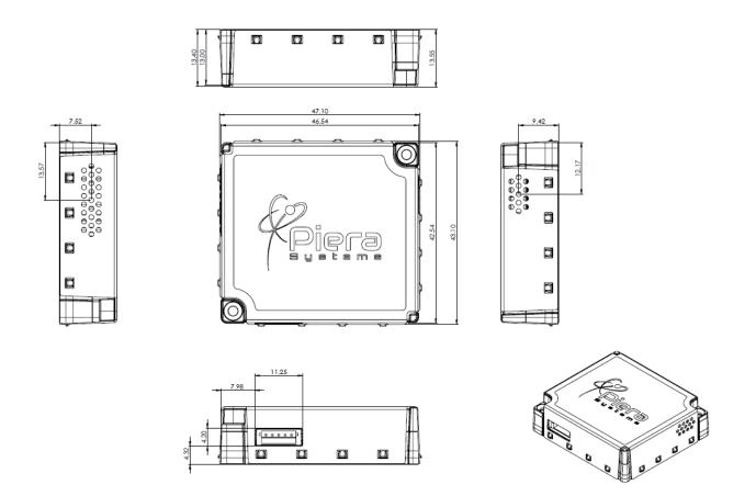
Any IPS models can be mounted by using two M2 screws.
