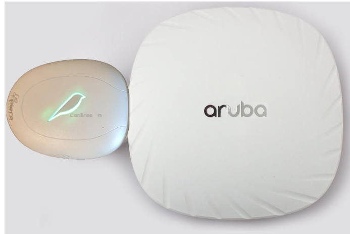
Figure 1: Canāree connected to USB Port on Aruba
