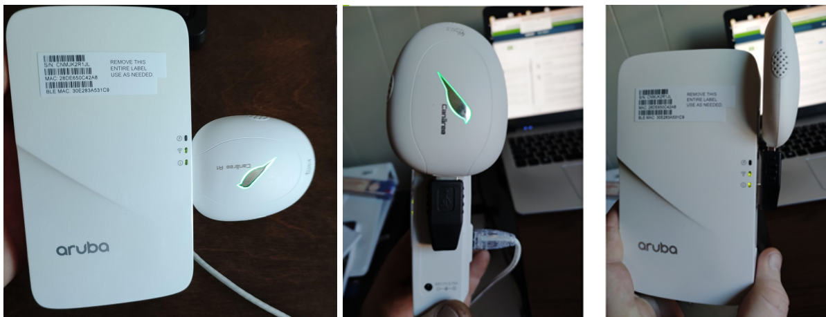
Figure X: A 90° USB Adapter is preferred on the Aruba 303 Model seen above.
