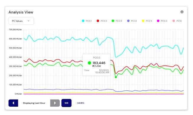
Figure 17. Analysis view showing Particle Count (PC) for all bins with PC0.5 selected at a specific time.
