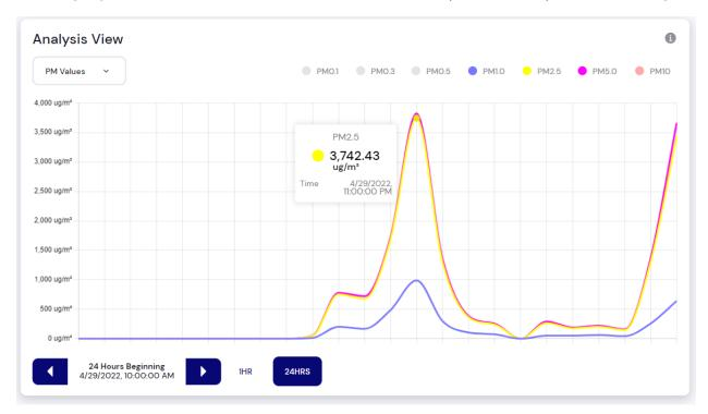
Figure 19. Analysis View showing Particle Mass (PM) Values over time PC2.5 highlighted
