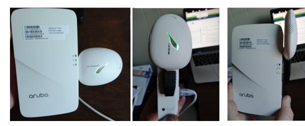
Figure X: A 90\* USB Adapter is preferred on the Aruba 303 Model seen above.
