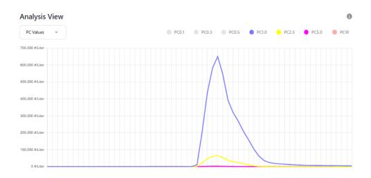
The figure above shows a candle burnt and quickly extinguished; within 1 ft of sensor; PC1.0 and above turned on in Analysis View
