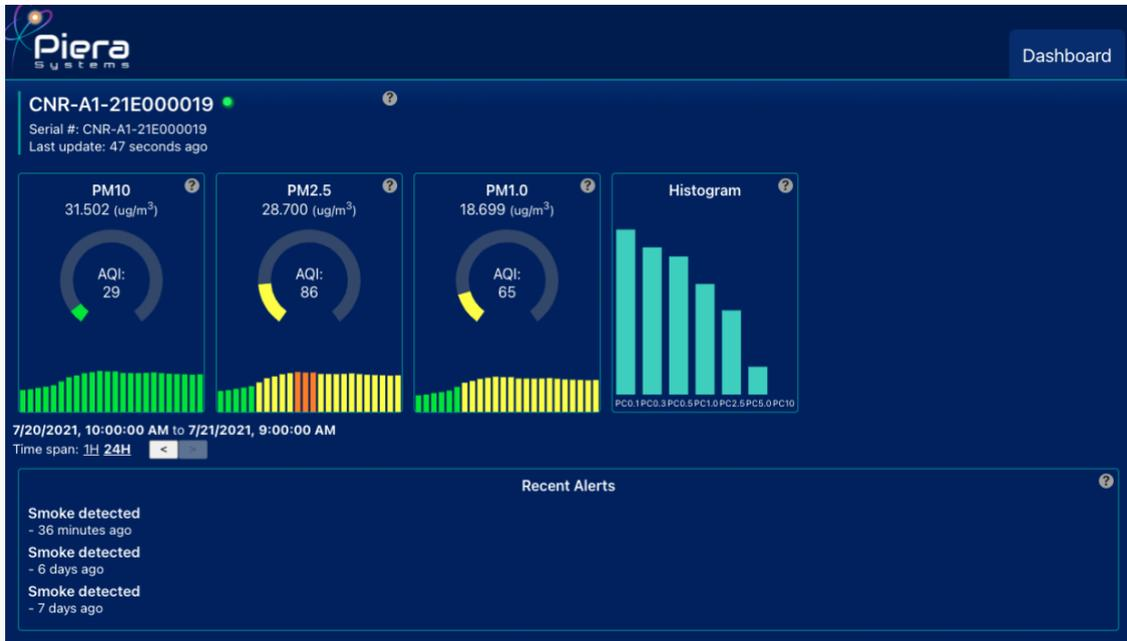
This morning at 9:15 AM I moved the Canāree and Sensirion outdoors. It detected a smoke event within minutes as all 3 PM values spiked with the majority being PM 1.0 and below.
