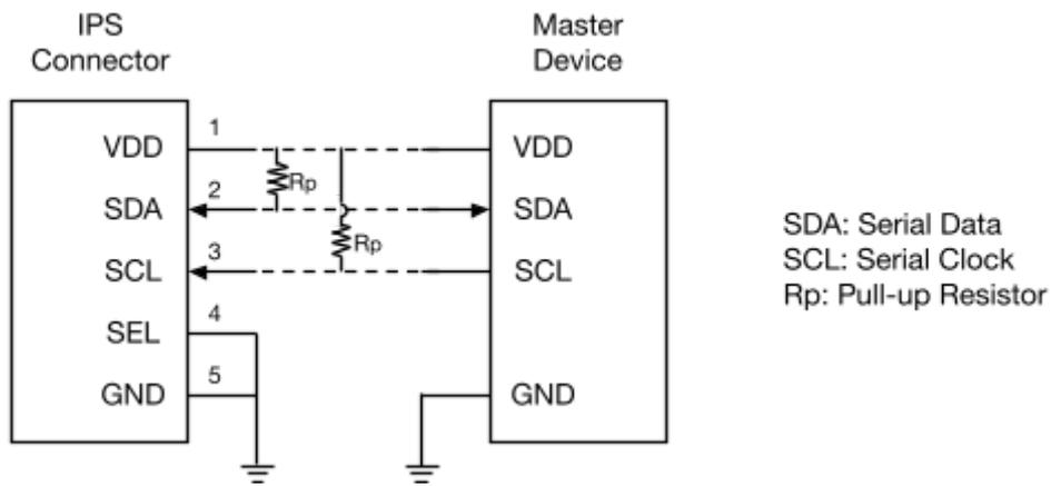
Fig. 4. Typical I<sup>2</sup>C interfacing
