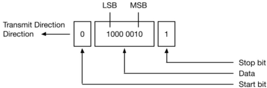
Fig. 2. UART (Universal Asynchronous Receiver Transmitter) data transfer
