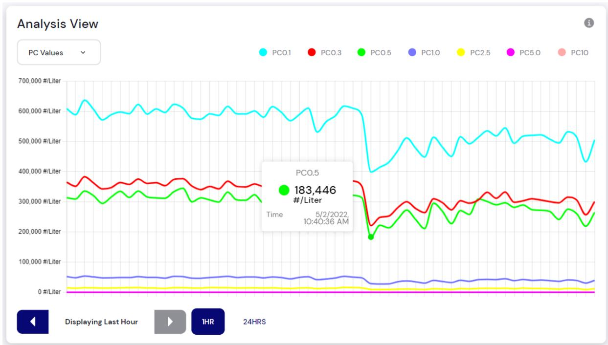
Figure 17. Analysis view showing Particle Count (PC) for all bins with PC0.5 selected at a specific time.
